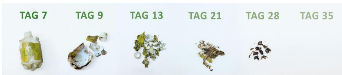
Composting of the bottle in industrial compost (at 60°C) within 35 days according to DIN EN 13432 (standard requires <90 days)
